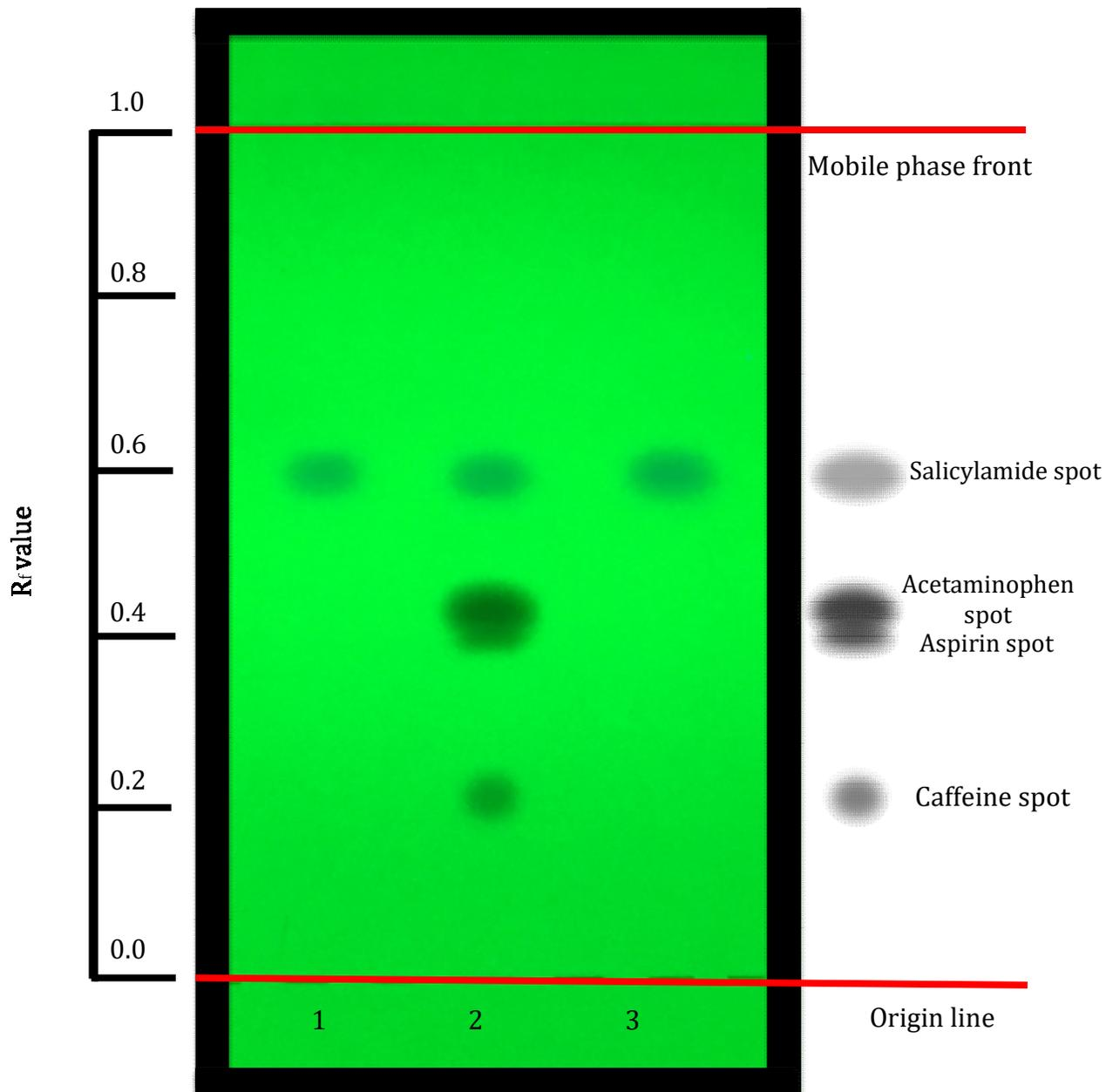
Plate observed under ultraviolet light at 254 nm
